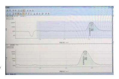
0 ppb, 1 ppb, 2 ppb, 5 ppb and 10 ppb chromium (VI) standard solutions were prepared for linear test. It can be seen from the following figure that the linear correlation coefficient is 0.9999, and the linear result is good.
